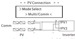
X1 series inverter support the following PV module connection modes.
